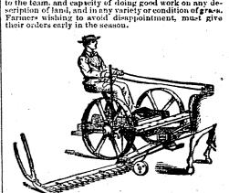
The Buckeye as a Reaper, The important advantages of the Buckeye as a Mover are retained in the Reager. The two driving wheels and flexible bar make it the ONLY Reaper perfectly adapted to uneven ground.
